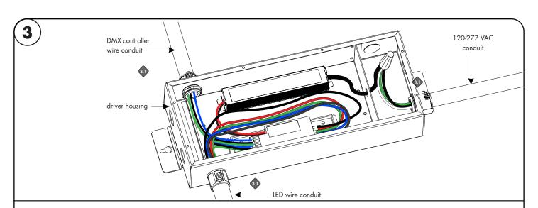
3.1 Insert the 120 - 277V AC power into the driver housing from the electrical panel. Followed by bringing 24V DC low voltage conduit one for the LED and other for the controller wires. Refer to diagram on page 2 to make all the proper wiring connections. Also, refer to page 3 to program decoder correctly.
